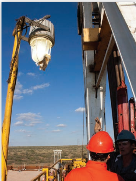
Workers discussing the danger of makeshift glare shields.
