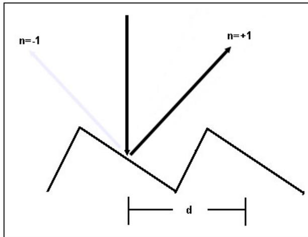
Unlike a CD though, astronomical reflection gratings have slots that are straight lines, and not circles. They are coated with a highly reflective material, to avoid losing light.
