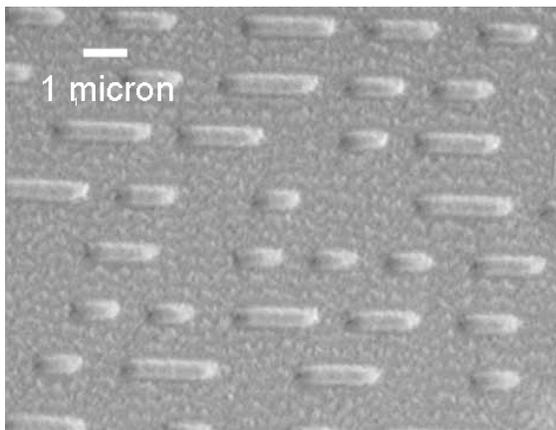
d. CDs are written with 650 nm (red) light beams. Is that consistent with the picture above?
