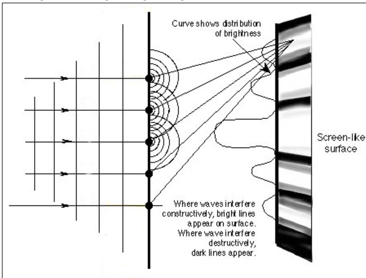
This diagram below shows how diffraction occurs through 'slits' (as opposed to the mesh 'grids' that are in the porthole). The general principles of diffraction and interference are the same in both cases.
