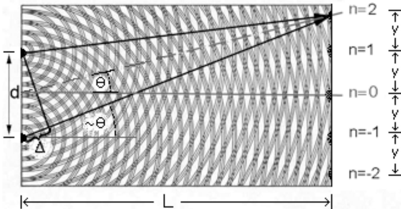
1. In the diagram above, a plane wave from left hits these two holes separated by a spacing “ $d$ ”, and is diffracted to the right. A dashed line marks the path toward the  $n=2$  spot, which is at an angle  $\theta$  away from the central spot. The spots on the screen are separated by a spacing “ $y$ ”. In this picture, the rings show the peak of the waves, and the separation of the rings is the wavelength  $\lambda$ .
