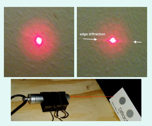
Diffraction from the edge of the card: At left above is the laser spot on the wall unobstructed, and at right is the spot on the wall when the laser beam is cut into by the card as shown below. This image shows the faint "spikes" that come from diffraction bending of light around the edge of the card.
