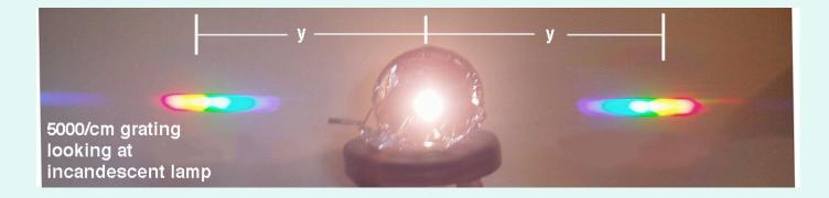
Appearance of incandescent lamp through the 5000/cm grating. The spots ("orders") are widely separated. Measure the order spacing by looking at one color.
