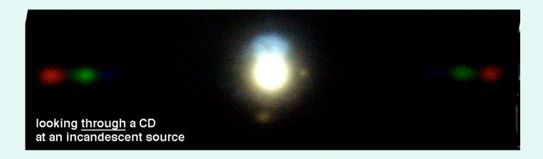
Appearance of incandescent lamp through a CD (compact disk). The spots ("orders") are widely separated, as for the 5000/cm grating. The ease with which these spots can be seen depends a lot on the CD. Do not use one with opaque labels. Disks with printed surfaces often allow enough light through to be viewed in this way.
