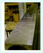
Grating at coudé focus of 2.7-m telescope and 1-m long echelon grating for EXES instrument (to fly on SOFIA)
