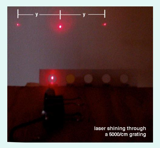
Same setup as in the previous slides, but with the 5000/cm grating. The spots now extend only in one direction, and are much more spread out.
