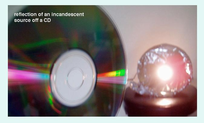
Diffraction is easily seen in reflected light off the surface of a CD, and produces the familiar iridescent appearance of these disks.
