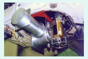
Medium resolution spectrograph on the Hobby-Eberly Telescope and CoolSpec at Cassegrain focus on the 2.7-m telescope. Both use diffraction gratings.
