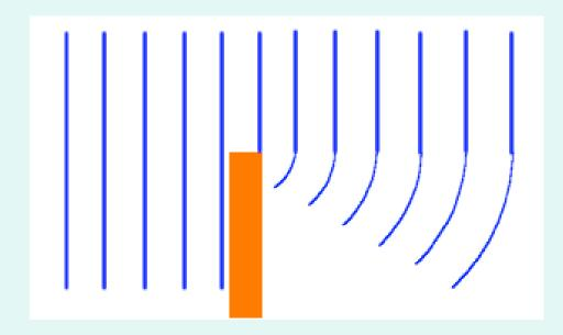
The waves bend around the barrier.
