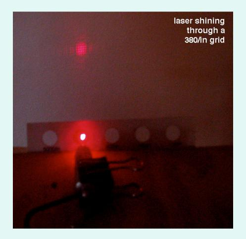
This shows the setup of the laser pointer shining at the Diffraction Materials Card that is taped to the edge of a table. The diffracted laser spot is projected on the far wall.
