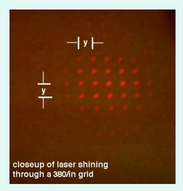
This shows a close-up of the projected laser beam with the setup laid out in the previous Annex slide. The diffracted spots are clearly visible. Projected on a piece of white paper, the spots can be marked for measurement.
