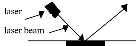
5. Using a pencil, trace the path onto the paper that the reflected laser beam follows. *Some methods of making the laser beam show up include a water spray bottle, dry ice (to make this really work put a small chunk of dry ice into hot water), or a commercial fogger. Baby powder or chalk dust will work too, but be careful if you have students with asthma or other respiratory problems.*
