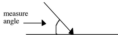
8. Using the protractor, measure the angle that the laser beam leaves the line at. This is called the **reflected angle**. Record this in a data table.
